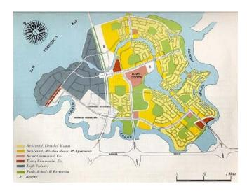
One of the more difficult aspects of the plan for the City was how to handle drainage in an area that was basically flat and at sea level. The engineering firm of Wilsey and Ham developed a plan to raise the surface level of the island four to five feet and to dig a central drainage basin area that also would serve as a runoff storage area. This drainage basin is now the Foster City Lagoon.
