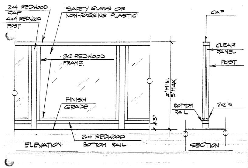
THE WIND SCREEN AS SHOWN IS PROVIDED AS A SUGGESTED DESIGN ONLY, AND MAY VARY AS LONG AS IT CONFORMS TO THESE GUIDELINES AND TO THE FOSTER CITY BUILDING CODES.
