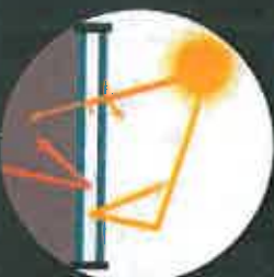
SunCoat Low-E allows most natural light to enter freely but reflects a significant portion of short-wave heat energy. In the summer, long-wave heat energy radiating from objects is reflected back outside, lowering cooling cost. In winter, internal long-wave heat energy is reflected back inside, lowering heating cost.
