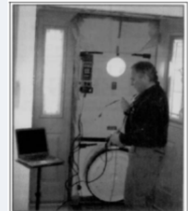
Photography: Abbott Dave Bunn, owner of Green Build Technology from Laramie, performs a blower door test on the second house built by students in the EWC Construction Technology program. The program uses environmentally-friendly building practices such as Energy Star and LEED.
